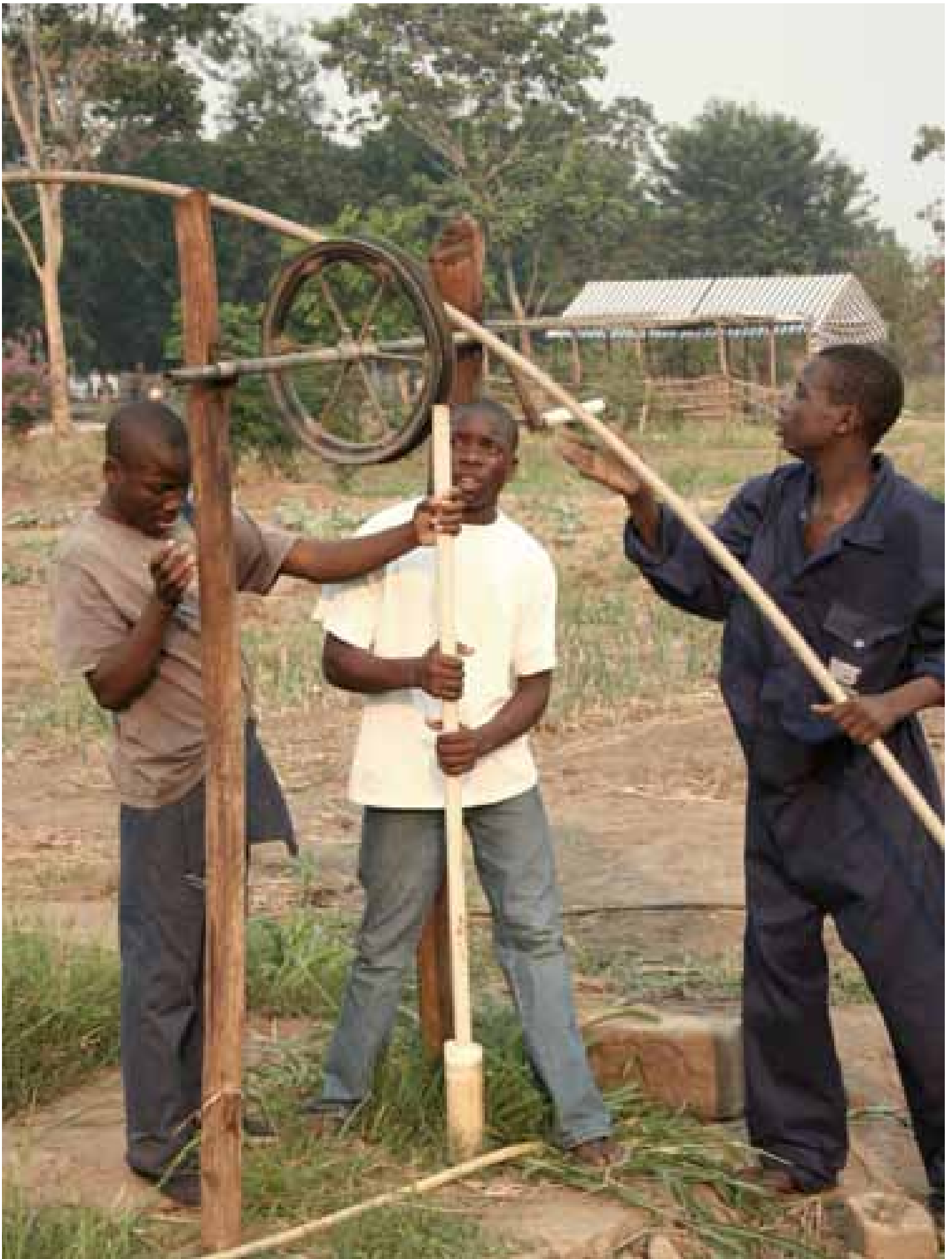
Vocational students learn to construct a hand-driven “rope pump” to provide reliable and affordable irrigation water.
